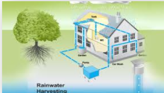
ROOF TOP RAINWATER HARVESTING
